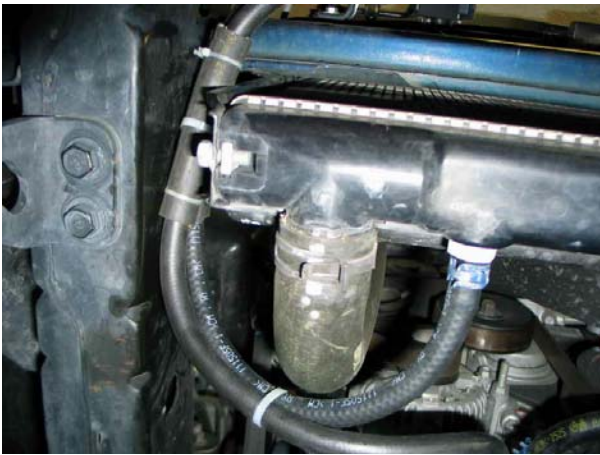
Picture 9. Protective sleeves on cooler lines as they pass between frame rail and radiator. Note zip ties holding hoses together.
