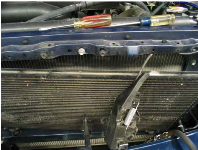
Picture 4. Condenser pulled forward to get access to the backside.
