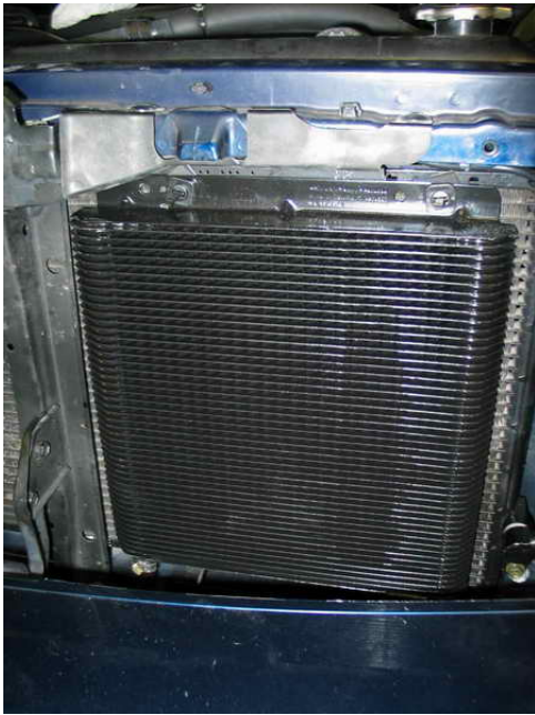
Picture 6. Cooler mounted.
