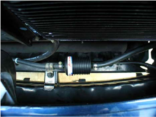
Picture 8. Filter installed right in front of cooler. Note line bracket mounted to factory trans cooler mounting boss.
