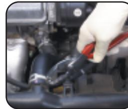
**5** DISCONNECT THE HOSE FROM THE FITTING – Twist the hose back and forth to loosen it. Pull firmly on the hose – it will be difficult to get started but should come off easily after being loosened. Be careful not to damage the flange.
